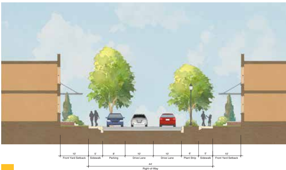
Fig 30. Street Section Proposed Baxter Court and Olmsted Court with one side of on-street parking and green stormwater infrastructure (New 44 ft. R.O.W.)
