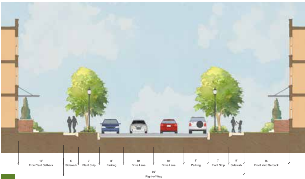
Fig 28. Street Section Existing North-South Streets with on-street parking and new green infrastructure (existing 60 ft. R.O.W.)
